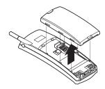
Place the SIM card onto its place. Make sure that the bevelled corner is top left and the gold contacts of the card face into the phone.
