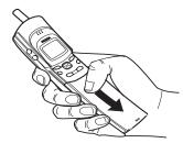
Closing the sliding cover ends or rejects a call. However, if you during a call press the left (Menu) and then close the sliding cover within a few seconds, the call is not terminated. Closing the sliding cover always exits the menu facility and memory functions.
